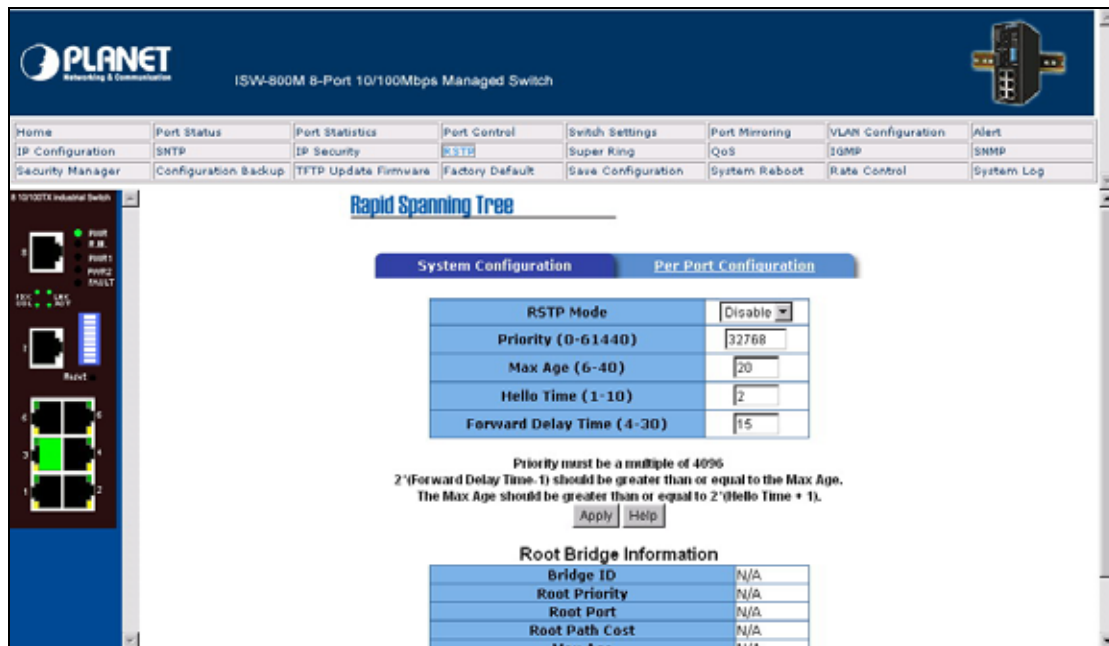
RSTP – System Configuration interface
